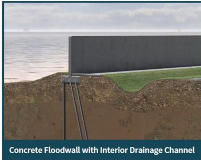
Concrete Floodwall with Interior Drainage Channel
